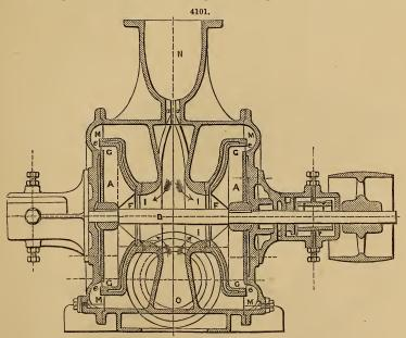
Centrifugal pumps are very serviceable when the height of ascension is not great. They possess the advantage of being adaptable to a varying discharge, and even a varying height, a change of velocity being all that is necessary to render them adequate to the case in question. They are easily
